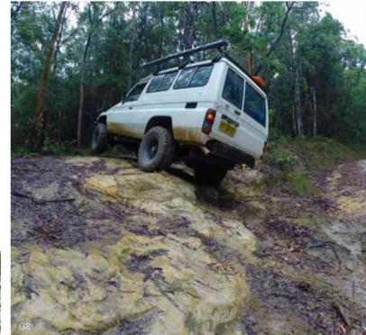
including vehicle weight and rim size, but, as a general guide, drop your tyre pressure to between 14-18 psi for sand driving and to around 25 psi for standard offroading on dirt tracks. Also remember to reinflate your tyres when you return to bitumen and/or fast speeds.
